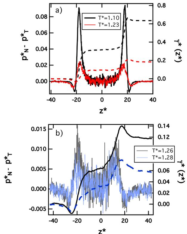
FIG. 4. Profiles of the difference  $p_N^*(z^*) - p_T^*(z^*)$  and  $\gamma^*(z^*)$  as a function of  $z^*$  for (a)  $T^* = 1.10$  and 1.23 and (b)  $T^* = 1.26$  and 1.28.
