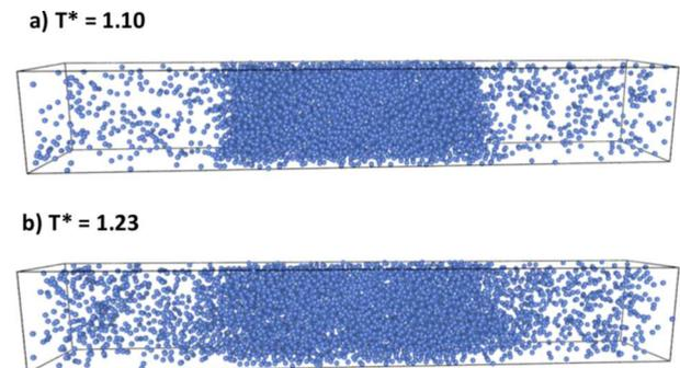
FIG. 2. Typical configurations of the liquid-vapor interface of the Lennard-Jones fluid at two reduced temperatures  $T^* = 1.10$  and  $T^* = 1.23$ .
