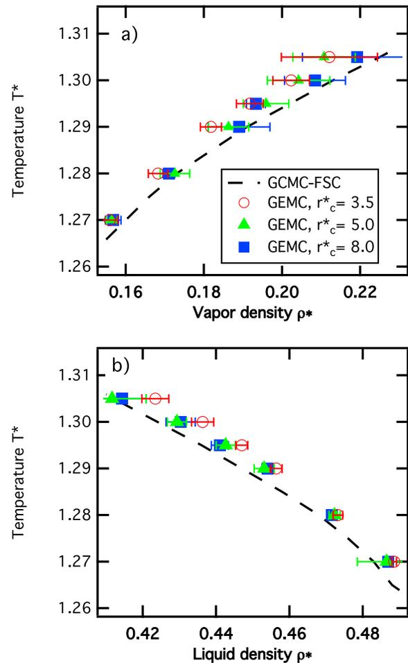
FIG. 8. Comparison between the (a) vapor and (b) liquid densities calculated with the GCMC-FSC<sup>33</sup> and GEMC<sup>36</sup> simulations.
