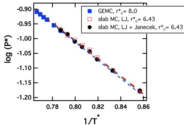
FIG. 9. Clausius-Clapeyron plots of the logarithm of the saturated vapor pressure as a function of the inverse temperature. For the GEMC simulations, we report the vapor pressure calculated with  $r_c^* = 8.0$ . For the slab simulations, the vapor pressures are calculated with  $r_c^* = 6.43$  by using the truncated LJ potential and the Janeček approach. The dotted lines show the Antoine fits.
