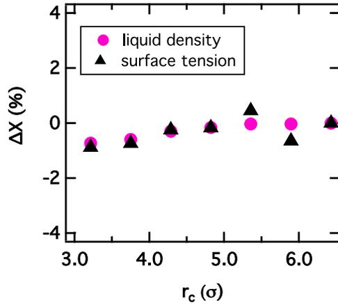
FIG. 1.  $\Delta X = 100 * [X(r_c) - X(r_{c,\text{full}})] / X(r_{c,\text{full}})$ ; the relative deviation calculated for the liquid density and surface tension at  $T^* = 0.84$  where  $r_{c,\text{full}} = 6.43 \sigma$ .
