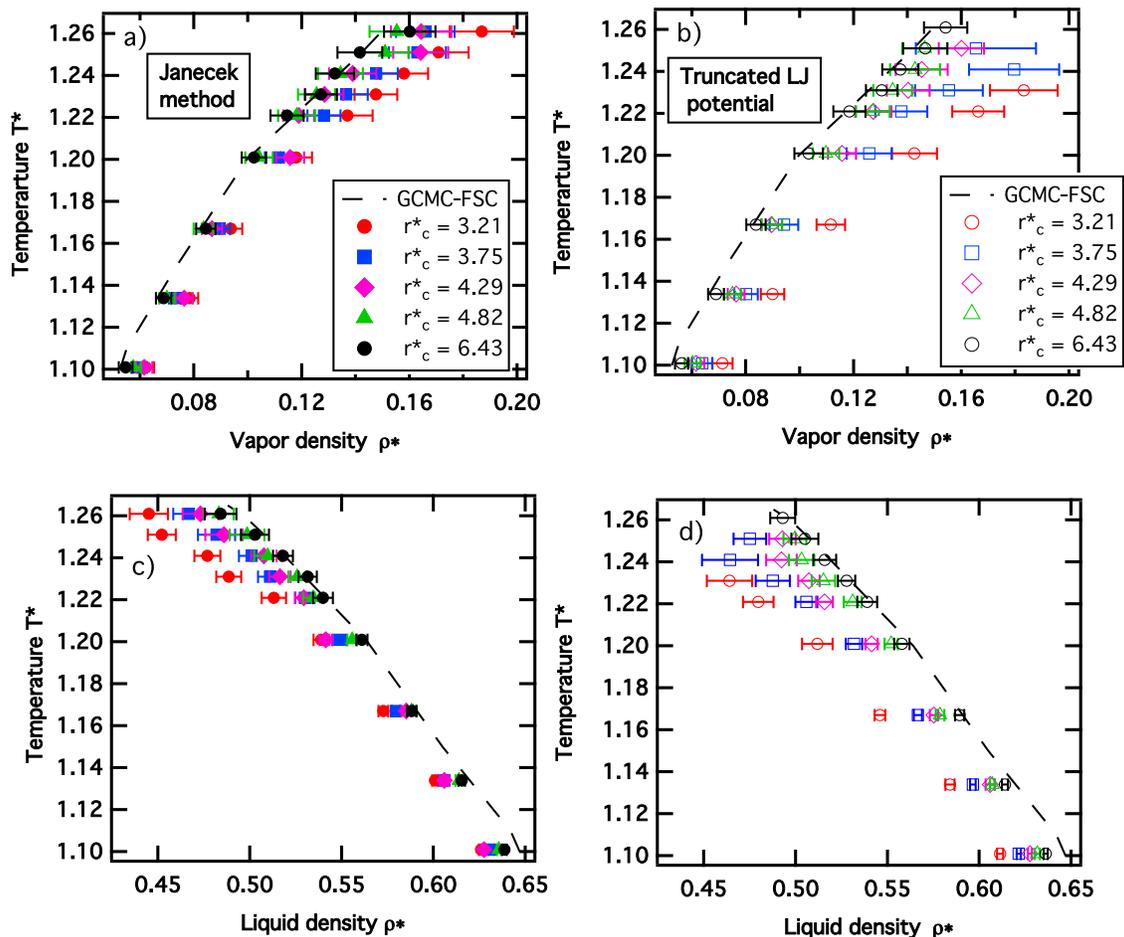
FIG. 5. Vapor (a) and (b) and liquid (c) and (d) densities calculated from the two-phase MC simulations at different reduced temperatures with both the slab-based tail Janeček method and the truncated Lennard-Jones potential model. The densities<sup>33</sup> calculated with the grand canonical Monte Carlo (GCMC) and the finite-size scaling (FSC) methods are given for comparison.
