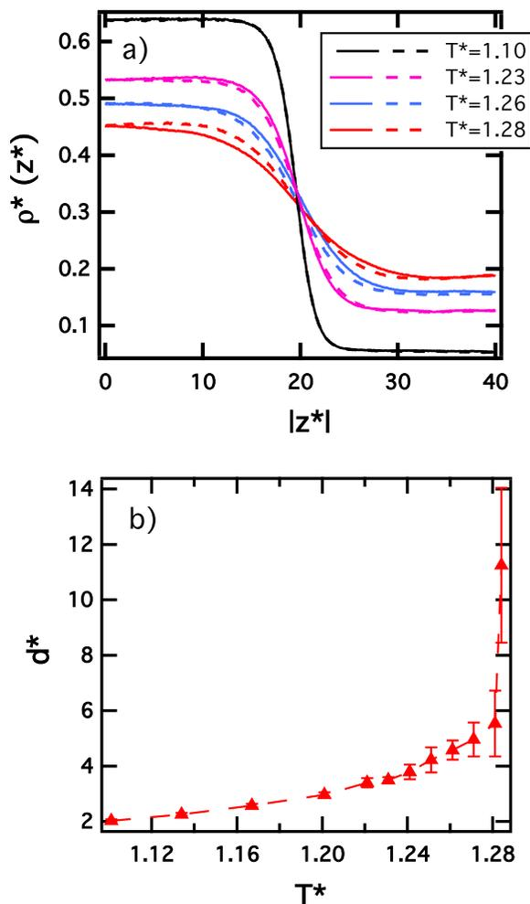
FIG. 3. (a) Superimposition of the density profiles of the LJ fluid at the liquid-vapor equilibrium calculated at four reduced temperatures. The left-hand sides of the density profiles are represented by solid lines and the right-hand sides by dotted lines; (b) calculated interfacial thickness at different reduced temperatures. The profiles and thickness of the interface are calculated with the Janeček method with a reduced cutoff of  $r_c^* = 6.43$ .
