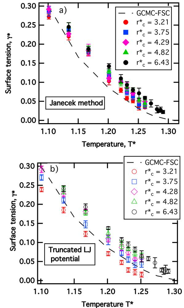
FIG. 6. The reduced surface tensions calculated in the critical region at different values of cutoff radius ( $r_c^*$ ) using the Janeček approach and the standard truncated LJ potential. The surface tensions<sup>33</sup> calculated with the GCMC-FSC methodology are given for comparison.
