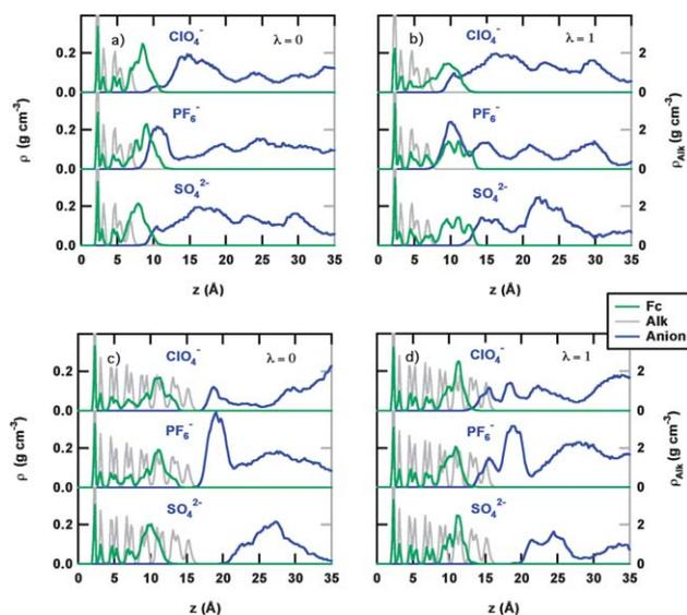
**Fig. 2** Molecular density profiles of the coadsorbed butanethiolate chains, ferrocenylhexanethiolate chain, and counterions as a function of the electrolyte anions for (a)  $\lambda = 0.0$  and (b)  $\lambda = 1.0$ . The same profiles are given in panels (c) and (d) where the dodecanethiolate chains replace the coadsorbed butanethiolate chains.
