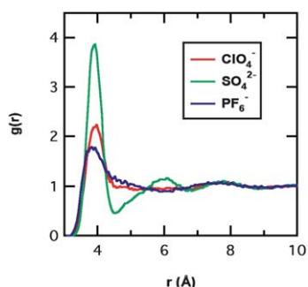
**Fig. 5** Computed anions- $\text{O}_w$  radial distribution functions in bulk conditions.  $\text{O}_w$  denotes the oxygen atom of water molecules.
