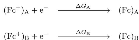
**Fig. 1** Redox reactions used to model the effect of the environment on the change in the redox properties of FcC<sub>6</sub>S–C<sub>4</sub>S–Au (System A represented by (Fc)<sub>A</sub>) and FcC<sub>6</sub>S–C<sub>12</sub>S–Au (System B represented by (Fc)<sub>B</sub>) SAMs.
