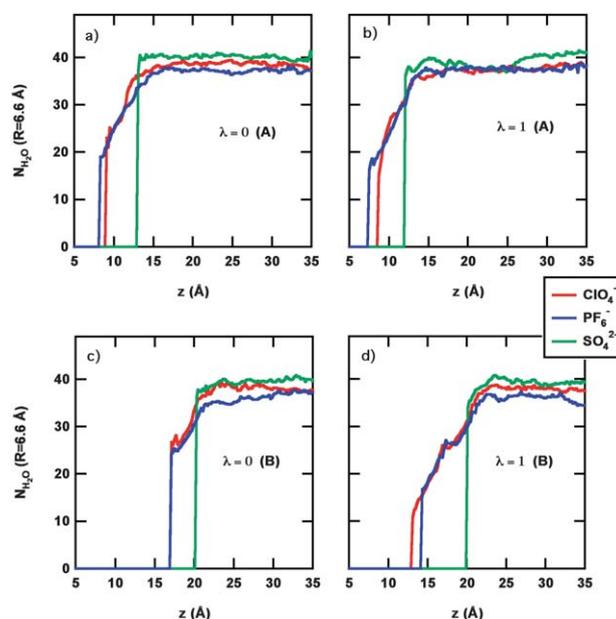
**Fig. 6** The profile of the number of water molecules as a function of  $z$  for each anion for system A at a)  $\lambda = 0.0$ , b)  $\lambda = 1.0$ . The same profiles are given in panels c)  $\lambda = 0.0$  and d)  $\lambda = 1.0$  for system B. The number of water molecules is calculated by integrating the RDF up to 6.6 Å.
