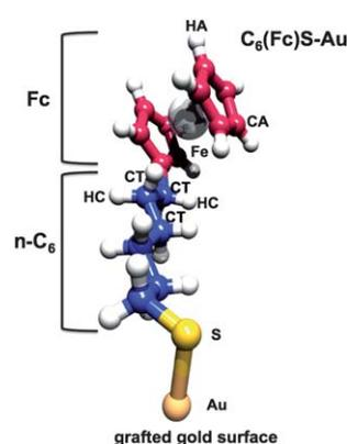
**Fig. 7** Labeling scheme of the ferrocenylhexanethiolate chain (FcC<sub>6</sub>S-Au) used in this work. The partial charges of the different atom types between the reduced and oxidized states are given in Table 7.
