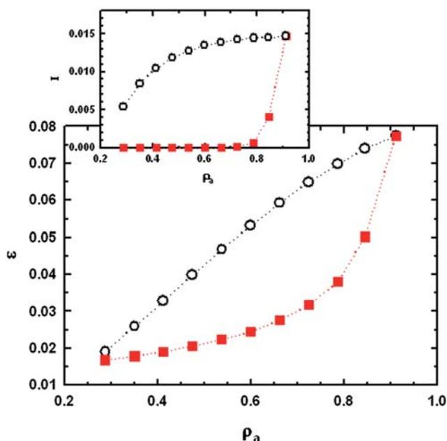
**Fig. 8** Friction coefficient  $\varepsilon$  as a function of the grafting density  $\rho_a$ . Open circles represent the reference systems, in which the missing polymer chains are replaced by solvent particles (see section 2.3). The inset shows the evolution of the brush interpenetration  $I$  for the same systems.
