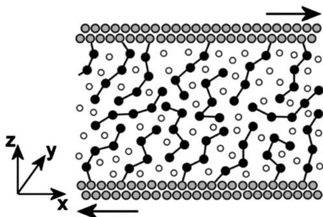
**Fig. 1** A schematic view of the simulated system. Grey circles are the wall particles tethered to a two-layers hexagonal lattice, black circles represent the polymer chains, and white circles represent solvent particles. The two arrows show the direction of the imposed shear movement of the surfaces along the  $x$ -axis.
