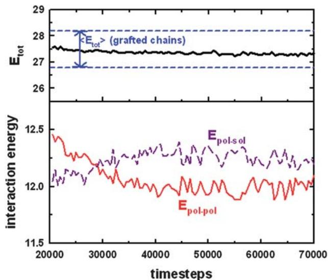
**Fig. 6** Average interaction energy of the detached chains as a function of time for the system with grafting density  $\rho_a = 0.474$ . The time scale is adjusted for each chain so that the detachment occurs at timestep 0. The total potential energy (top) and the polymer–polymer and polymer–solvent conservative contribution (bottom) are shown.
