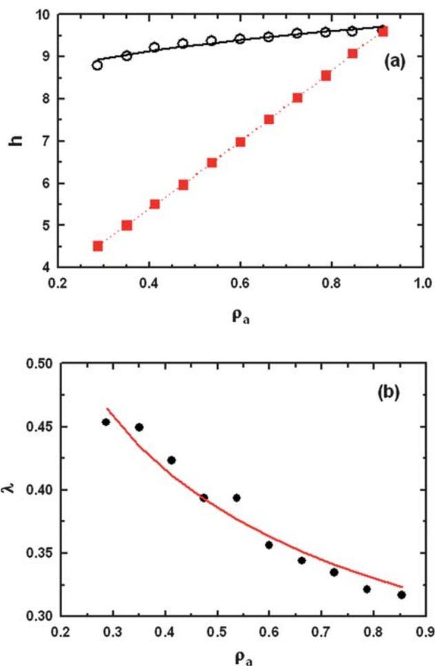
**Fig. 4** (a) Brush height  $h$  as a function of the grafting density  $\rho_a$  in the middle of the box. Open circles represent the reference systems, in which the missing polymer chains are replaced by solvent particles (see section 2.3). (b) Penetration length of the polymer solution inside the brush  $\lambda$  as a function of  $\rho_a$ .
