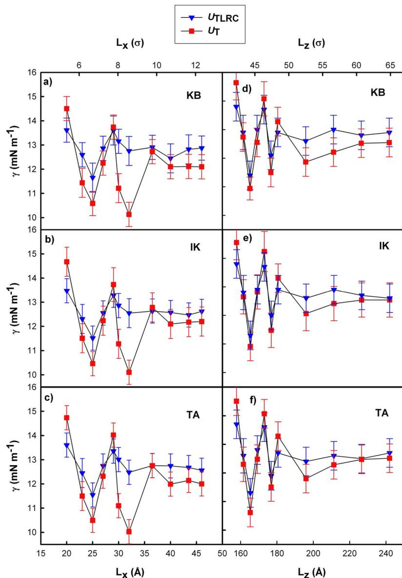
FIG. 1. (Color online) Total surface tension values ( $\text{mN m}^{-1}$ ) calculated with respect to the  $L_x$  and  $L_z$  dimensions from MC simulations using the  $U_{\text{TLRC}}$  and  $U_T$  potentials. The bottom  $x$  axis is labeled in angstroms and the top  $x$  axis in units of  $\sigma$ . The surface tension is calculated from the virial route (KB and IK) and from the thermodynamic route (TA) as indicated in the different curves.
