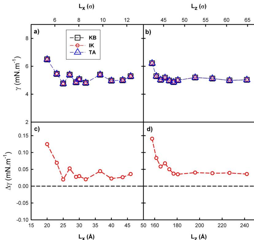
FIG. 5. (Color online) (a) and (b) Surface tension values ( $\text{mN m}^{-1}$ ) calculated as a function of (a)  $L_x$  and (b)  $L_z$  dimensions for KB, IK, and TA approaches. Stress anisotropy ( $\text{mN m}^{-1}$ ) as a function of (c)  $L_x$  and (d)  $L_z$  dimensions. All these calculations have been performed using the spline potential  $U_{\text{sp}}$ . The error bars are smaller than the symbols.
