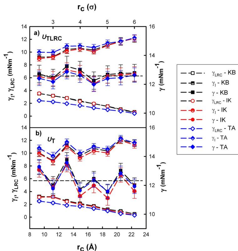
FIG. 6. (Color online) Intrinsic ( $\gamma_i$ ) and LRC ( $\gamma_{\text{LRC}}$ ) contributions to the surface tensions (left axis) and total surface tension ( $\gamma$ ) (right axis) as a function of the cutoff radius calculated with (a) the  $U_{\text{TLRC}}$  potential and (b) the  $U_T$  potential. The error bars of the LRC parts of the surface tensions are smaller than the symbols.
