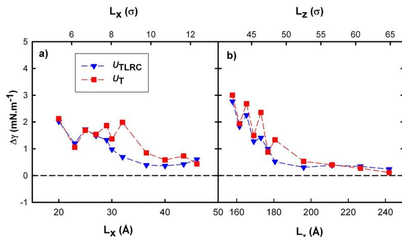
FIG. 4. (Color online) Stress anisotropy  $\Delta\gamma$  ( $\text{mN m}^{-1}$ ) as a function of (a)  $L_x$  and (b)  $L_z$  for  $U_{TLRC}$  (triangle) and  $U_T$  (square) potentials.
