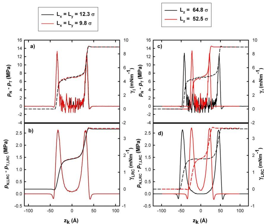
FIG. 3. (Color online)  $p_N - p_T$  pressure profiles calculated for (a) two different interfacial areas and (c) two different  $L_z$  dimensions;  $p_{N,LRC} - p_{T,LRC}$  profiles calculated for (b) two different interfacial areas and (d) two different  $L_z$  dimensions. The integrals of the  $p_N - p_T$  profiles are plotted in the right axis.
