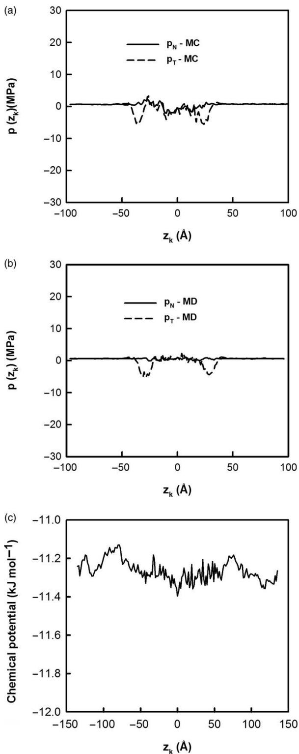
Figure 3. Normal and tangential pressure components calculated in the liquid–vapour interface of the *n*-pentane at  $T = 325$  K from (a) MC and (b) MD using a LJ potential and a force changed by a cubic spline function. (c) Total chemical potential of the liquid–vapour interface of methane at  $T = 120$  K calculated from MC simulations using a LJ potential changed by a cubic spline function.
