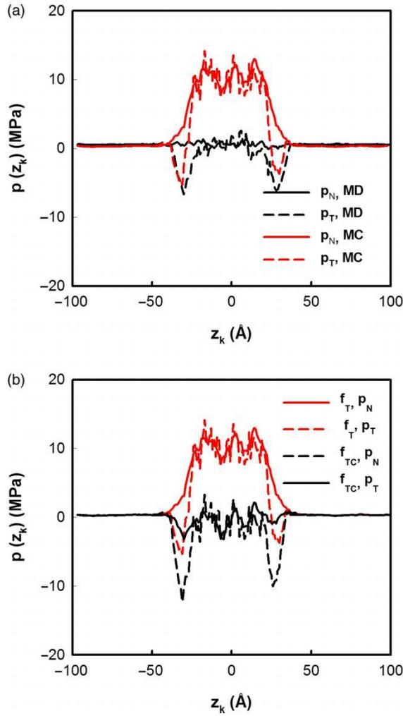
Figure 2. Normal and tangential pressure components calculated in the liquid–vapour interface of the *n*-pentane at  $T = 325$  K from (a) MC using a truncated potential and MD using a truncated force and (b) MC using both a truncated force  $f_T$  and a truncated force modified by an additional impulse  $f_{TC}$ .
