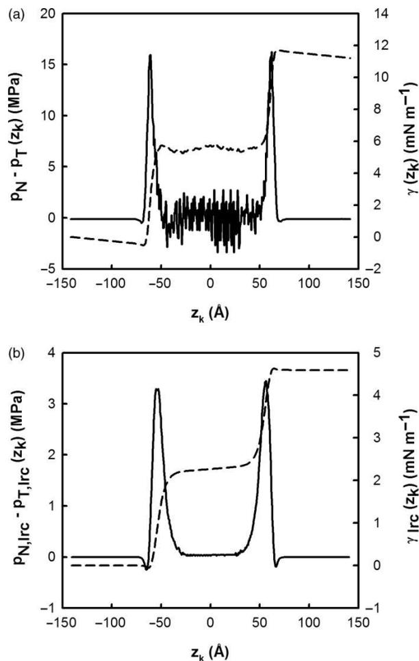
Figure 4. (a) Difference between the normal and tangential pressure profiles for the liquid–vapour interface of the  $n$ -pentane at  $T = 300$  K; (b) difference between the normal and tangential components of the LRCs to the pressure tensor. On the right axis, the integral of each difference is plotted as a function of  $z$ .
