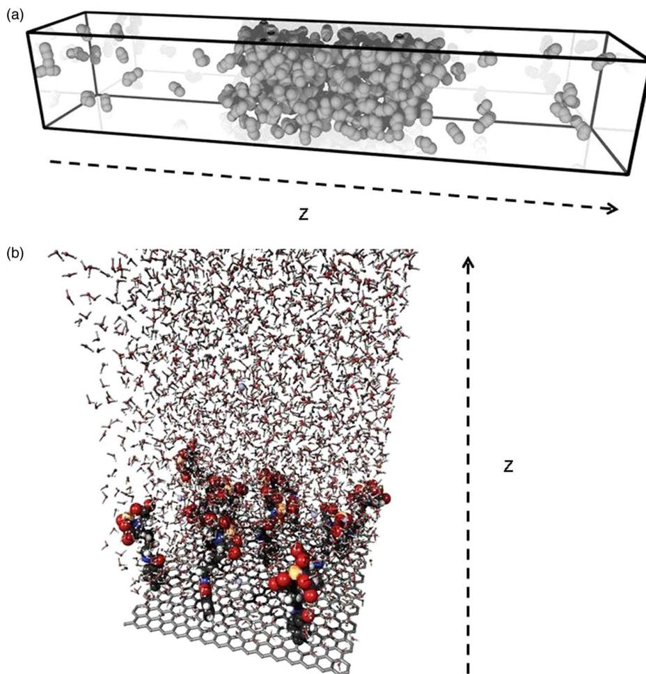
Figure 1. (a) Configurations of the *n*-pentane liquid–vapour interface at  $T = 350$  K. (b) Snapshot of a MD configuration of 10 grafted NTA-Cu(II) complexed onto the HOPG surface with the water molecules.
