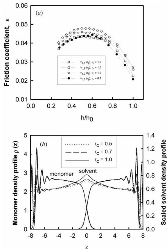
Figure 6. (a) The friction coefficient profiles calculated for each of the three conservative potential forms and for a smaller size of solvent particle ( $r_c = 0.5$ ). (b) The monomer and solvent density profiles calculated for three sizes of solvent particles.
