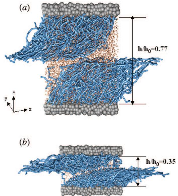
Figure 1. Typical configurations for the polymer brushes system in good solvent conditions under shear at two surface separations. (a)  $h/h_0 = 0.77$  and (b)  $h/h_0 = 0.35$ . The polymer chains are represented using sticks and the open circles represent solvent particles. The grafted surfaces are represented by bigger grey open particles.
