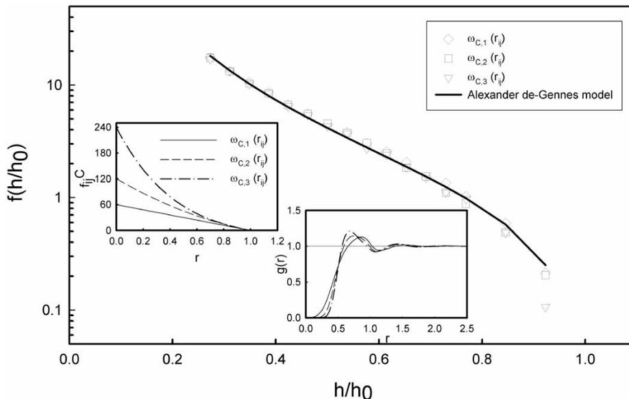
Figure 5. The normal force-compression profiles calculated in polymer brushes using the different forms of the conservative potential. The leftmost inset shows the shape of the conservative force and the rightmost the corresponding pair correlation function  $g(r)$  for a pure DPD fluid with the different conservative potentials.
