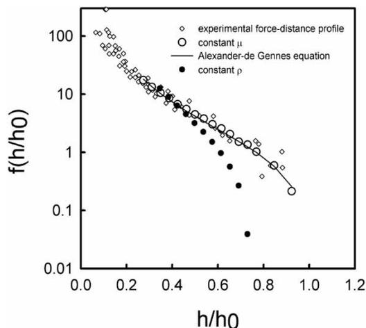
Figure 3. A semi-log plot of the experimental and simulated force-compression profiles. The solid line represents the profile calculated from the Alexander-de Gennes equation. The experimental and theoretical results have been shifted vertically to obtain the best agreement with the simulated data.
